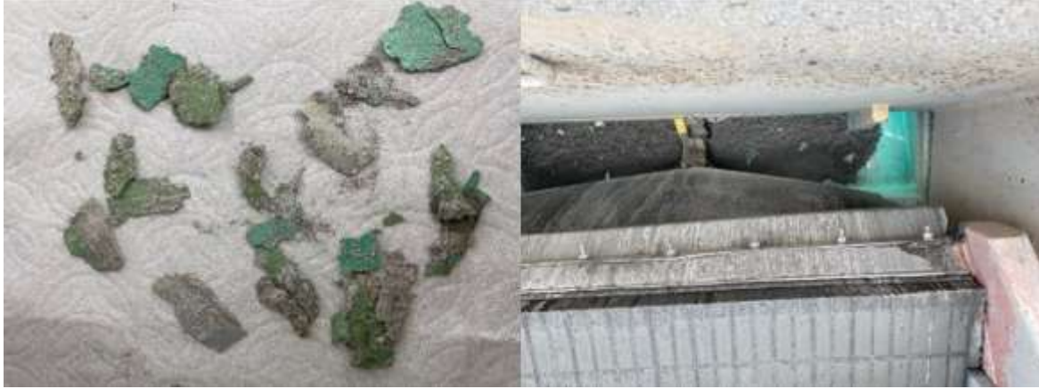
Figure 7: Coating pieces caught by the mud loggers
